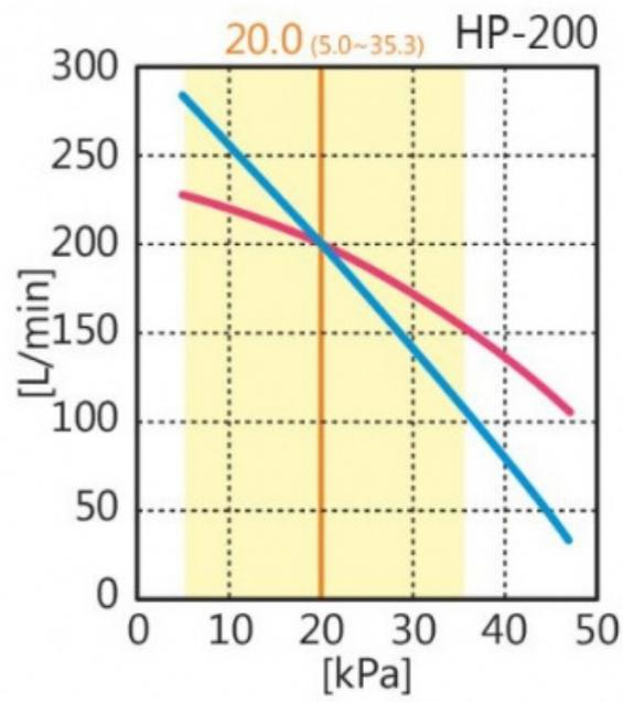
— 50Hz — 60Hz — Rated pressure — Pressure range for use
