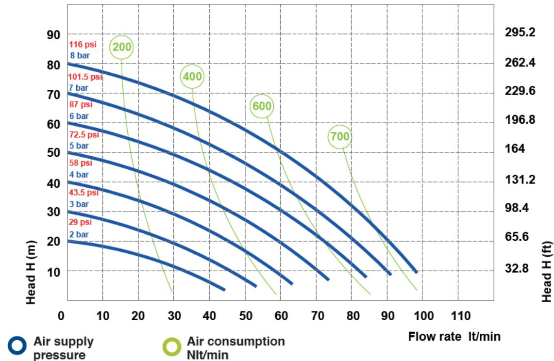
The curves and performance values refer to pumps with submerged suction and free delivery outlet, with water at 20°C. These data may vary according to the construction materials and hydraulic conditions.
