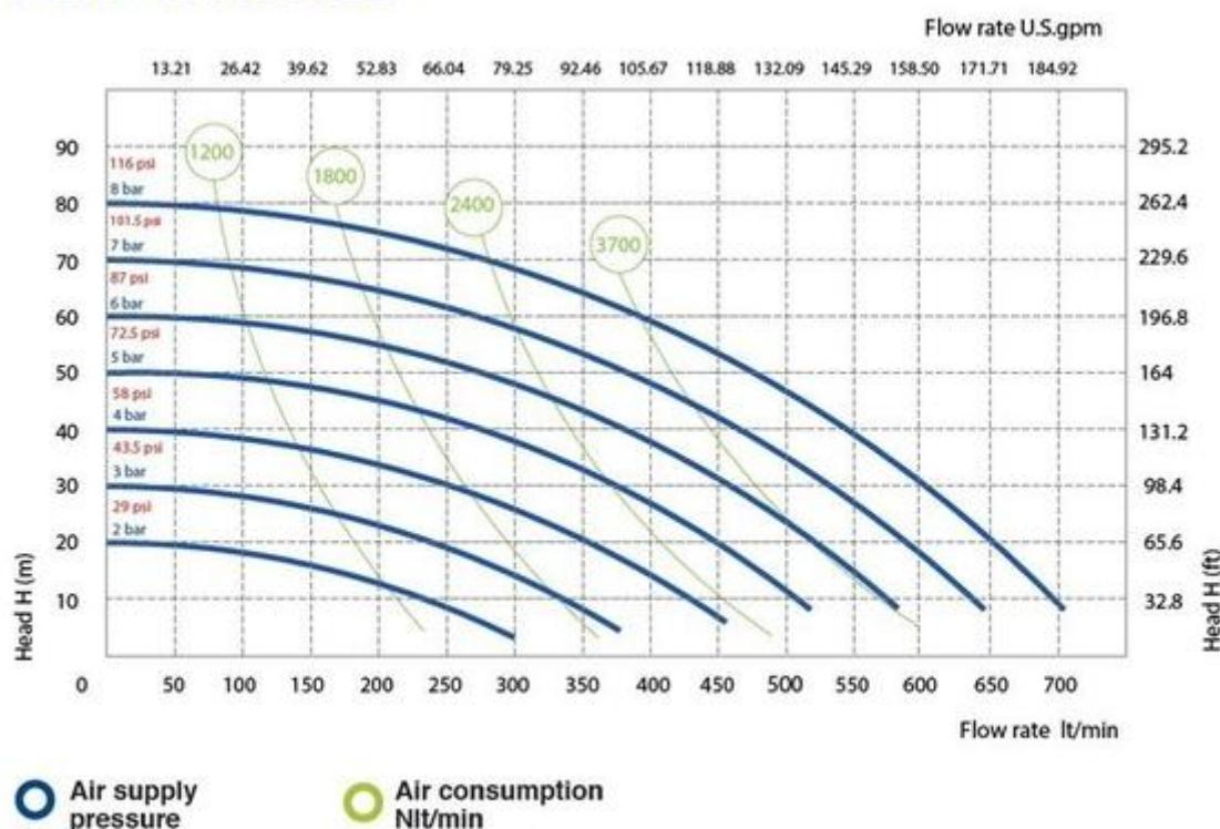
The curves and performance values refer to pumps with submerged suction and a free delivery outlet with water at 20°C, and vary according to the construction material.
