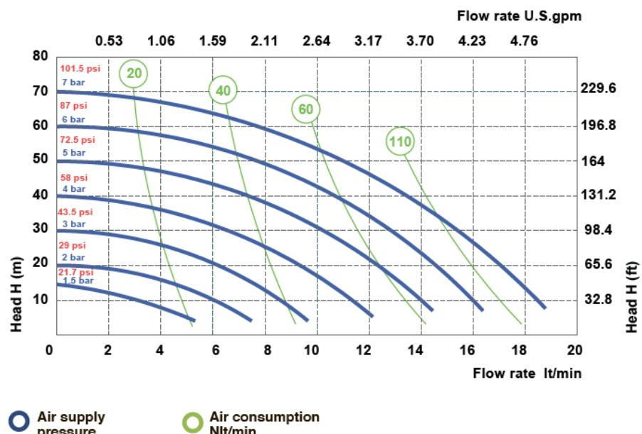
The curves and performance values refer to pumps with submerged suction and free delivery outlet, with water at 20°C. These data may vary according to the construction materials and hydraulic conditions.
