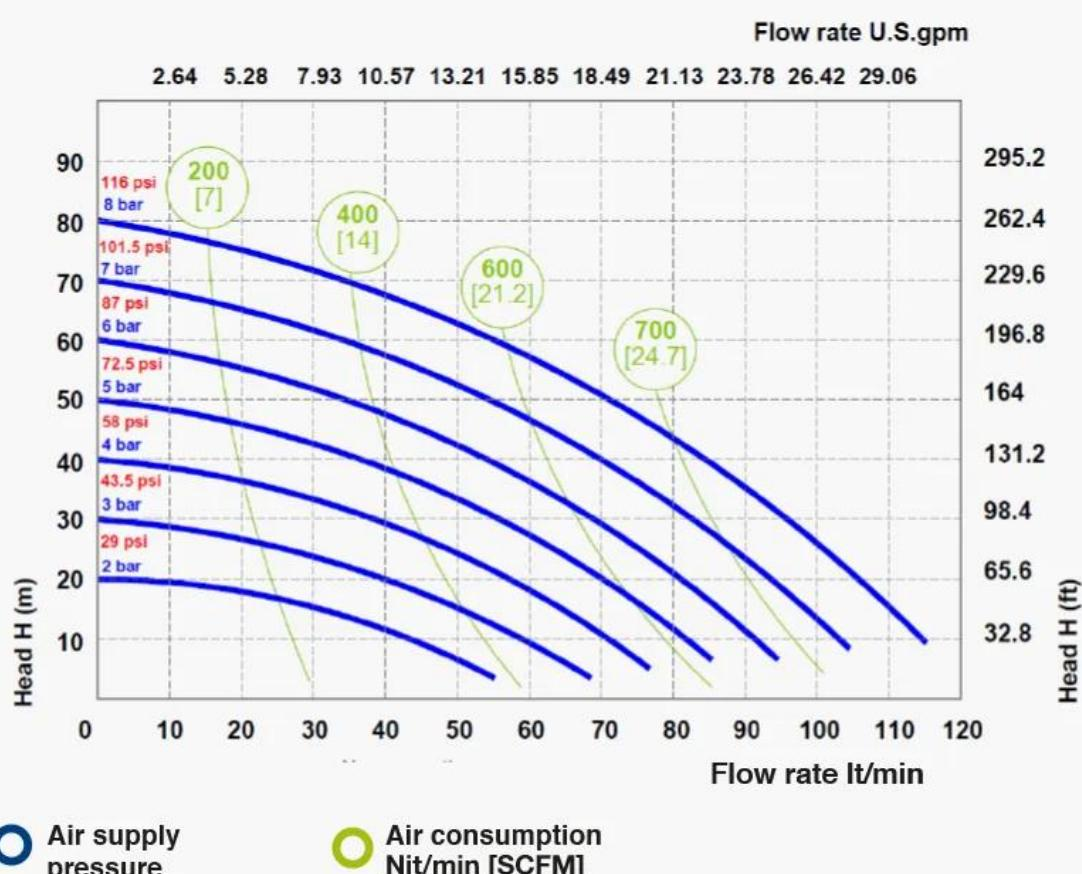
The curves and performances refer to pumps with immersed suction and free-mouth delivery, with water 20°C, and vary depending on the construction material and hydraulic conditions.
