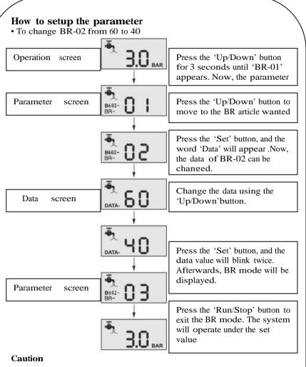
Before setting the parameter, please refer to the parameter table to check the articles that can't be changed during operation for protection of the pump.
