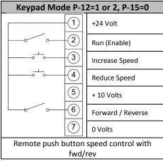
By default if the enable signal is present the drive will not Enable until the START button is pressed. To automatically enable the drive when the NOTE enable signal is present set P-31 = 2 or 3. This then disables the use of the START & STOP buttons
