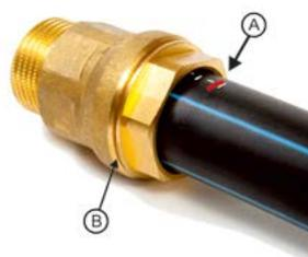
Tighten the nut until the nut flange is touching the body (B). When a reinforcement is used, the nut may remain approximately 1mm away from the frame.
