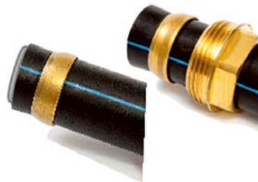
The front part of a properly tightened ring will bend symmetrically onto the pipe. When a reinforcement is used, the ring will penetrate slightly deeper into the pipe because it won't back off. The connection can always be undone and retightened in the same spot provided that the ring is scratch-free. If the connection has to be undone often (for instance in case of water pumps), the seal can be proofed by wrapping a few layers of PTFE tape around the ring.
