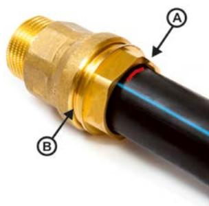
Do not unscrew the nut (B). Push the pipe to the bottom of the connector, all the way to the marking (A) on the pipe. When tightening the connector, make sure the pipe stays fully inserted.
