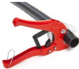
Cut the pipe straight across, remove all burr and bevel the outer edge of the pipe (HELA chamfering tool #8059010).
