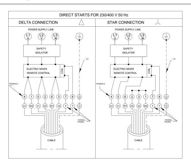
For  $Y - \Delta$  starting, use electrical motor cables following the instructions of control panel electrical scheme.
