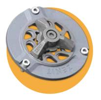
The heart of the models **GRG** is an effective, entirely redesigned **cutting device** which consists of a plate with sharp-edged holes and as a shaving, rotating triangular knife, attached to the impeller, both of which are made of **X 102 CrMo 17 KU martensitic steel**.
