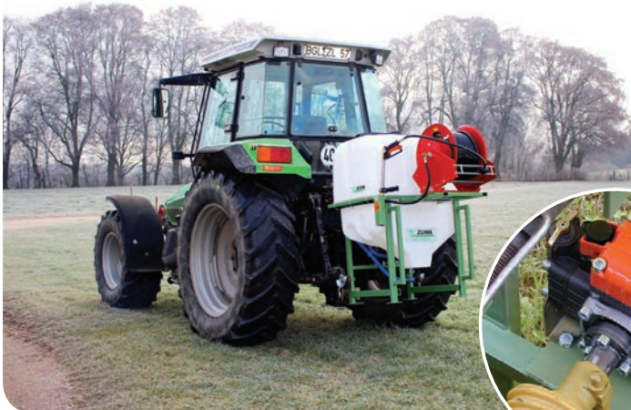
diaphragm pump with p.t.o. connection
