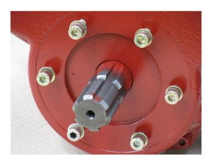
If the pump is going to be driven by a hydraulic motor, check the oil flow and pressure of the circuit needed to make turn the pump at a turning speed as close as possible to the nominal turning speed of the pump, and never quicker.
