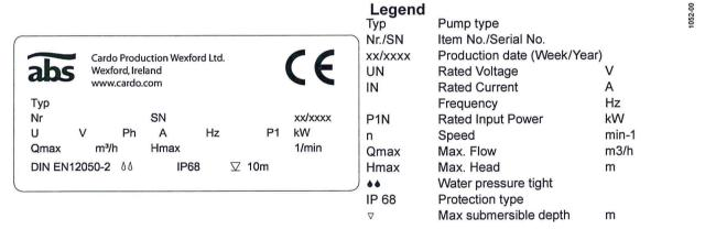
Figure 1 Nameplate Standard Version
