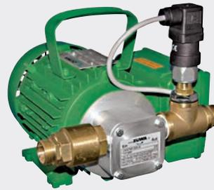
The pressure switch shuts off the pump when reaching a preset pressure level. As soon as the pressure drops again by 30% the pump automatically starts anew. Device just works with 400 V motor.
