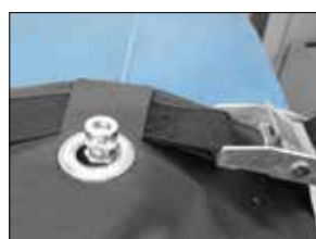
Detail of the quick installation system of the hoses on the tool mouth
