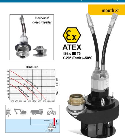
SP36 ATEX is a 3" hydraulic waste pump for clear and heavily loaded liquids, impeller and shell are made in stainless steel. The pump produce high performance thanks to hydraulic power and the exclusive closed single channel impeller which allows very high efficiency with flow rates up to 1600 L / min, head up to 50 meters.
