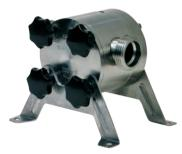
For easy opening of the pump by hand without using tools. For this operation it is not necessary to remove the pump from its installed position. This provides an easy access for cleaning, inspection and maintenance. (for NIROSTAR A and B)
