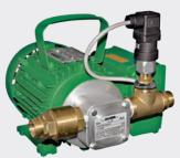
The pressure switch shuts off the pump when reaching a preset pressure level. As soon as the pressure drops again by 30% the pump automatically starts anew. Device just works with 400 V motor.
