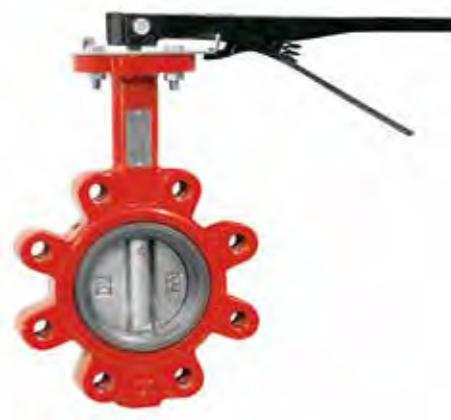
Interception butterfly valve LUG type, with threaded ears, complete with operating lever up to DN100 and hand-wheel for larger diameters. The limit switch for monitoring the ON/OFF valve are available on request.
