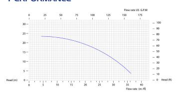
The curves and performance values refer to pumps with free delivery outlet with water at 20  $^{\circ}$ C, and two poles motor 50 Hz. These data may vary according to the construction materials and hydraulic conditions.
