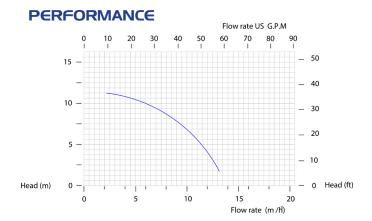
The curves and performance values refer to pumps with free delivery outlet with water at 20 °C, and two poles motor 50 Hz These data may vary according to the construction materials and hydraulic conditions.
