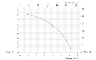
The curves and performance values refer to pumps with free delivery outlet with water at 20 °C, and two poles motor 50 Hz. These data may vary according to the construction materials and hydraulic conditions.
