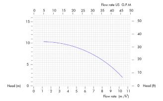
The curves and performance values refer to pumps with free delivery outlet with water at 20  $^{\circ}$ C, and two poles motor 50 Hz. These data may vary according to the construction materials and hydraulic conditions.
