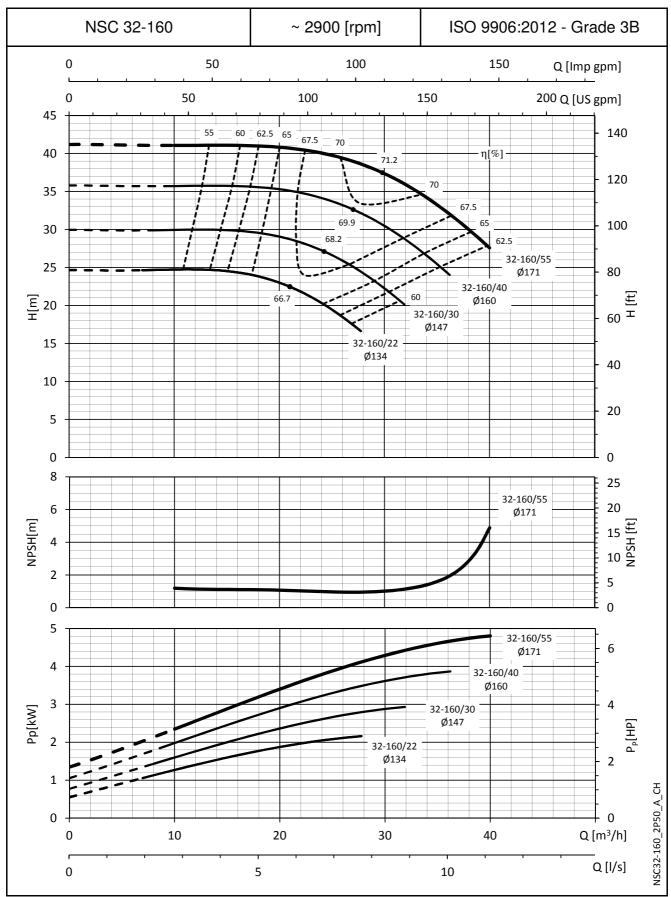
The NPSH values are laboratory values; for practical use we suggest increasing these values by 0,5 m. These performances are valid for liquids with density  $\rho=1$ ,0 Kg/dm³ and kinematic viscosity  $\nu=1$  mm²/sec.
