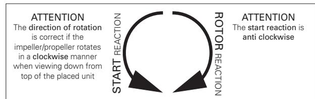
With bigger pumps the check may be done by watching the rotation of the impeller through the discharge or suction inlet. Switch the pump on and off and check the direction of rotation when the impeller rotates slowly.
