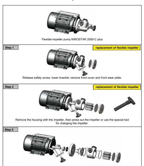
Remove the rear wear plate and the screws of the cylinder head, remove the cylinder head itself and withdraw the mechanical seal
