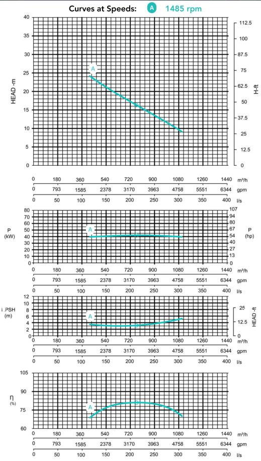
Note: Pump power P include mechanical seal friction and bearing frame losses, from a run in bearing frame. (Testing according ISO 9906:2012-38)
