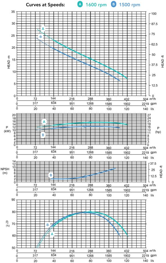
Note: Pump power P include mechanical seal friction and bearing frame losses, from a run in bearing frame. (Testing according ISO 9906:2012-38)
