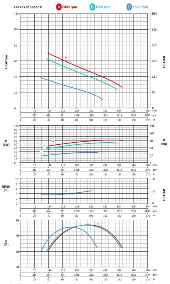
Note: Pump power P include mechanical seal friction and bearing frame losses, from a run in bearing frame.
