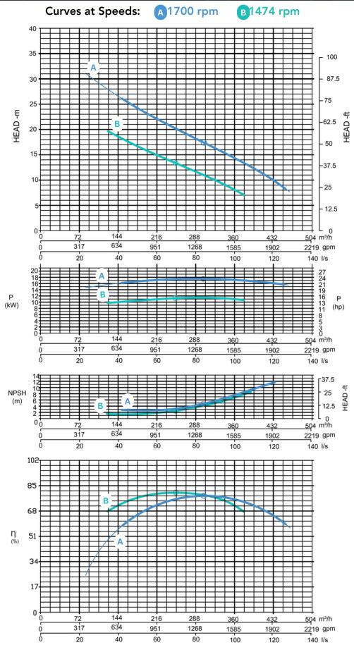
Note: Pump power P include mechanical seal friction and bearing frame losses, from a run in bearing frame. (Testing according ISO 9906:2012-38)
