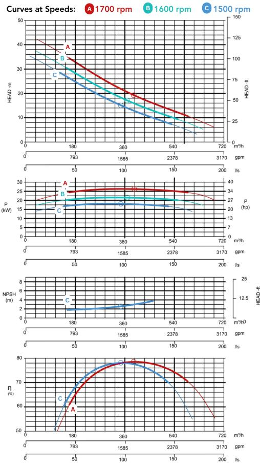
Note: Pump power P include mechanical seal triction and bearing frame losses, from a run in bearing frame. (Testing according ISO 9906:2012-38)
