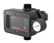
Grundfos PM PLUS is a pressure manager designed for automatic start/stop control of Grundfos or other pumps for water supply in domestic applications. With adjustable start pressure, PM PLUS can easily be customised to your specific application. PM PLUS features automatic protection that stops the pump in case of water shortage, preventing dry running. In case of temporary power outage, PM PLUS automatically resets itself once power is restored.
