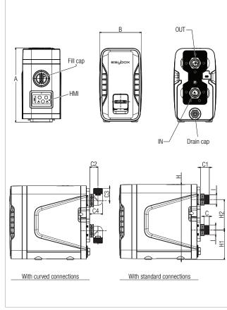
Two pairs of fittings will be supplied, both elbow and standard.
